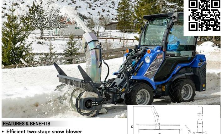
Heavy duty frame and transmission with replaceable cutting edge
